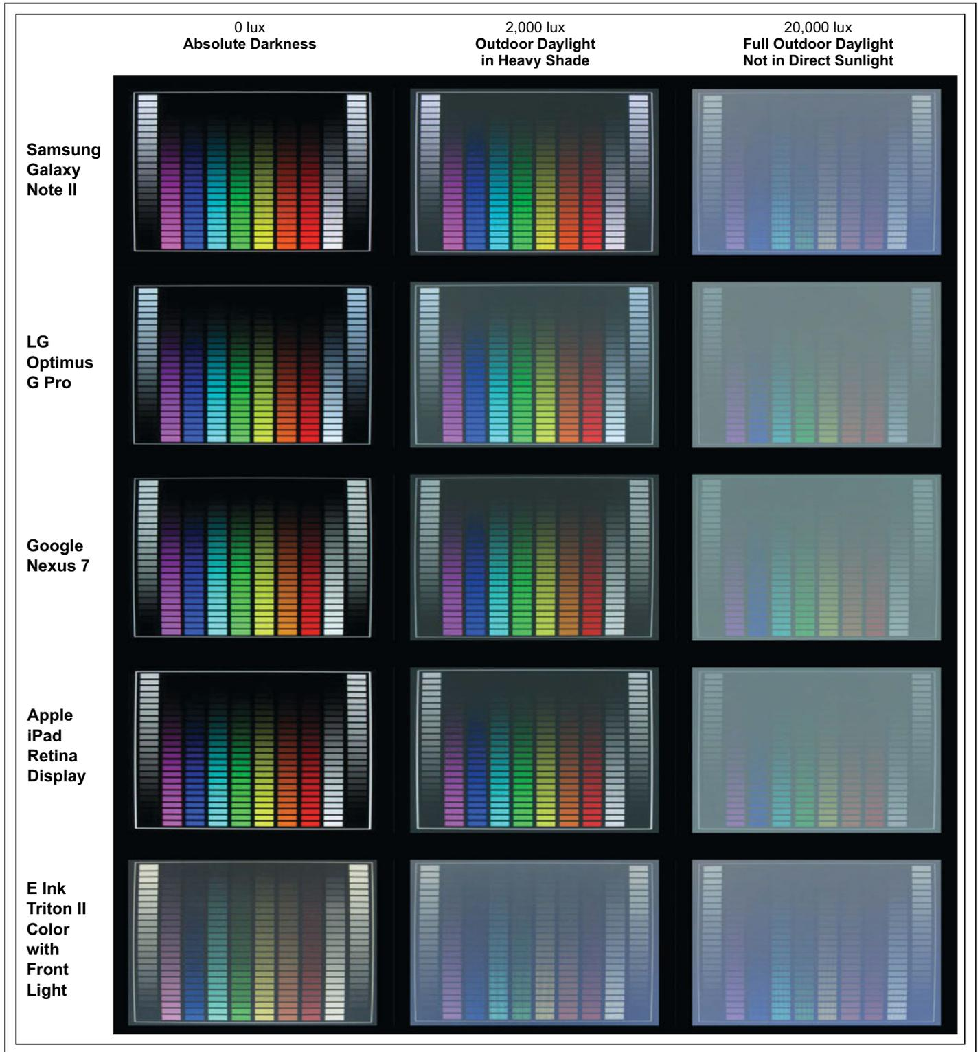
*Fig. 5: Shown are tablet screen shots in high ambient light. Because of the wide range of ambient light levels and screen reflectance values, the screen shots were taken with a camera set for automatic exposure. As a result, the exposure levels vary between the tablets, but that is also the same way that our eyes would process each image. All of the photos were taken at the display's maximum brightness setting.*
