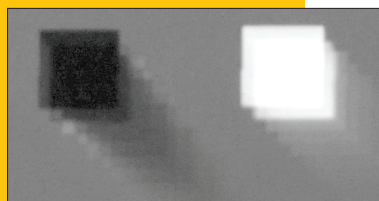
The screen on the left was grabbed from a motion speed test of 1,093 pixels per second, with the black and white squares indicating real-world pixel response times of 60ms and 40ms, respectively. The screen on the right shows the same lengthy response times during a faster test of 1,609 pixels per second.
